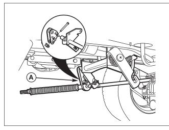
Figure 18. Lift Arm Extension A. Lift Bracket
